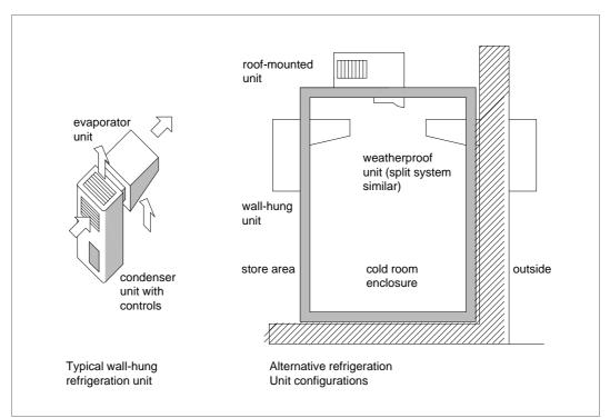
Figure 3: Packaged refrigeration units
