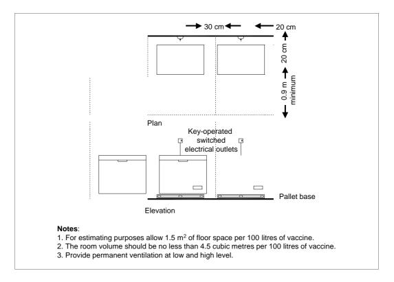
Figure 7: Refrigerator and freezer layout
